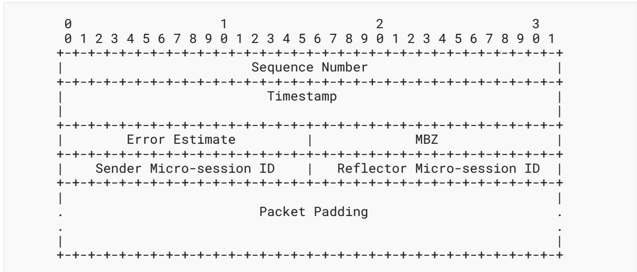
Figure 2: Micro Session-Sender Packet Format in Unauthenticated Mode
