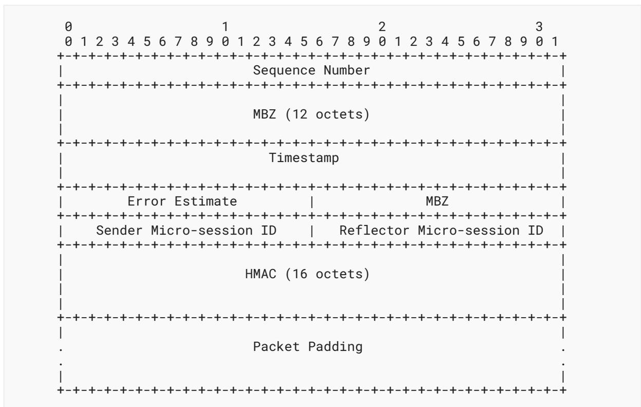
Figure 3: Micro Session-Sender Packet Format in Authenticated Mode
