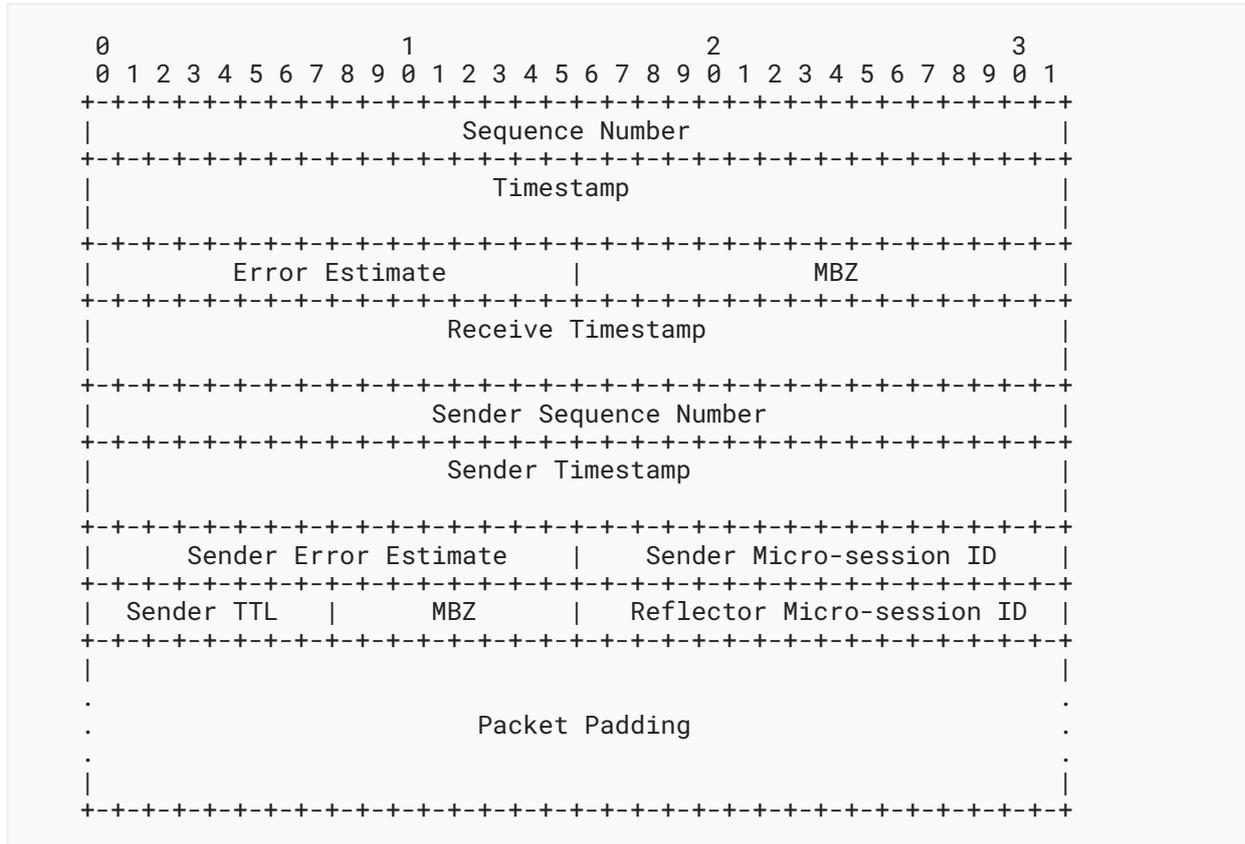
Figure 4: Micro Session-Reflector Packet Format in Unauthenticated Mode
