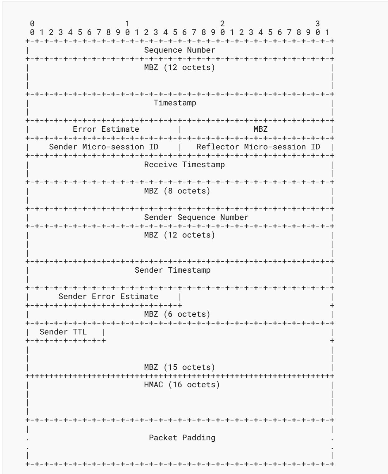
Figure 5: Micro Session-Reflector Packet Format in Authenticated Mode
