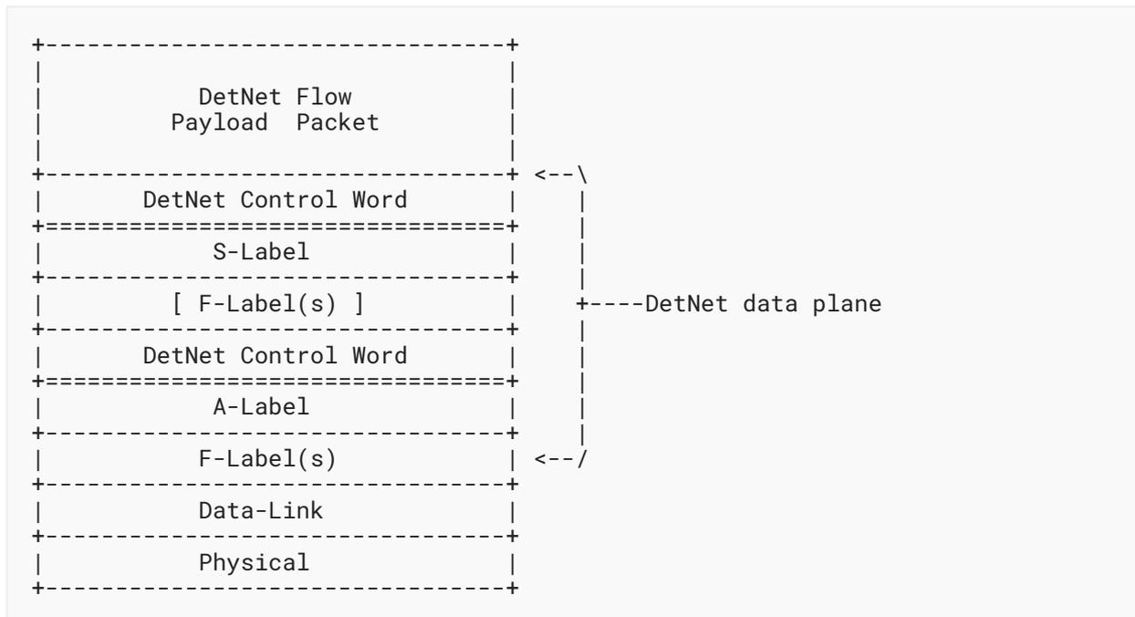
Figure 6: DetNet Aggregation as a New DetNet Flow
